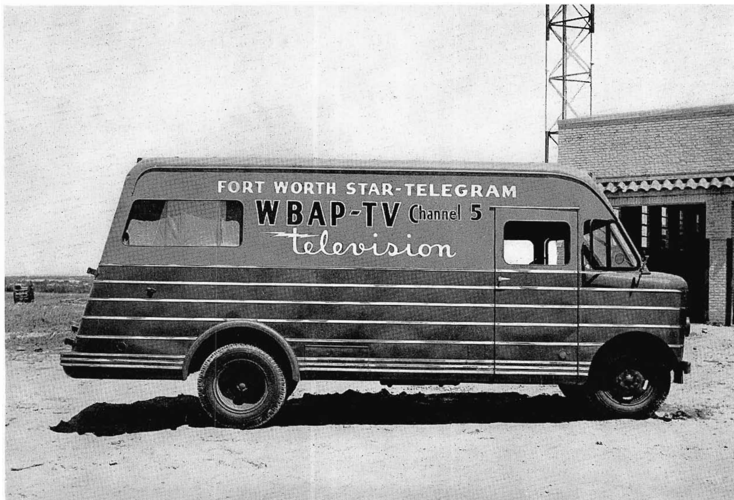
FIG. 21. WBAP-TV's field unit is an RCA TV-50A Mobile Unit with complete equipment, including RCA TK-30A Cameras and RCA TTR-1A Microwave Relay Equipment.
