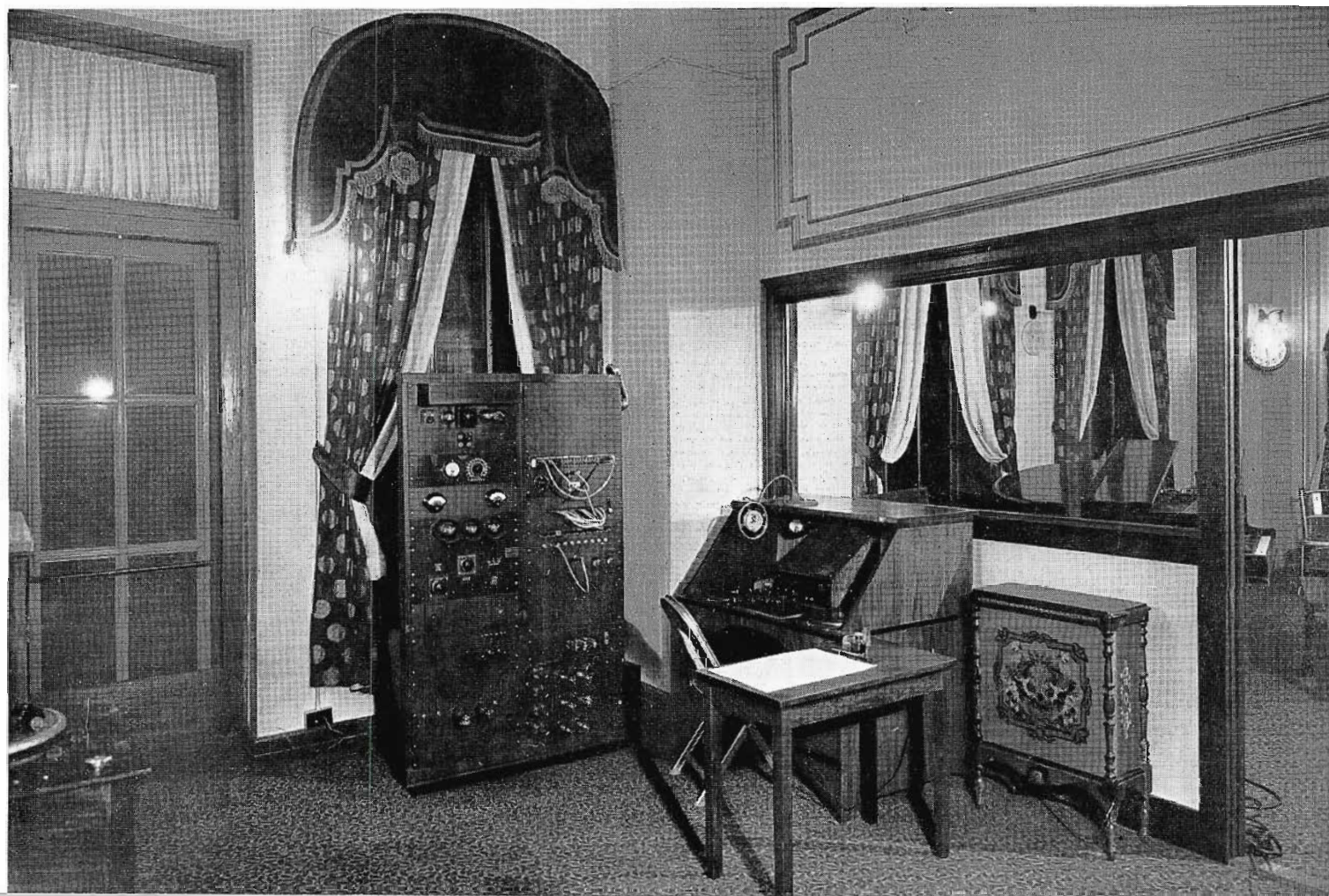
FIG. 13. This 100-watt control room, shown in the Hotel Claridge around 1931, had as its only commercial equipment the RCA 12-A amplifier, 600-A carbon microphones, and a 106-B speaker. All other equipment was composite.
