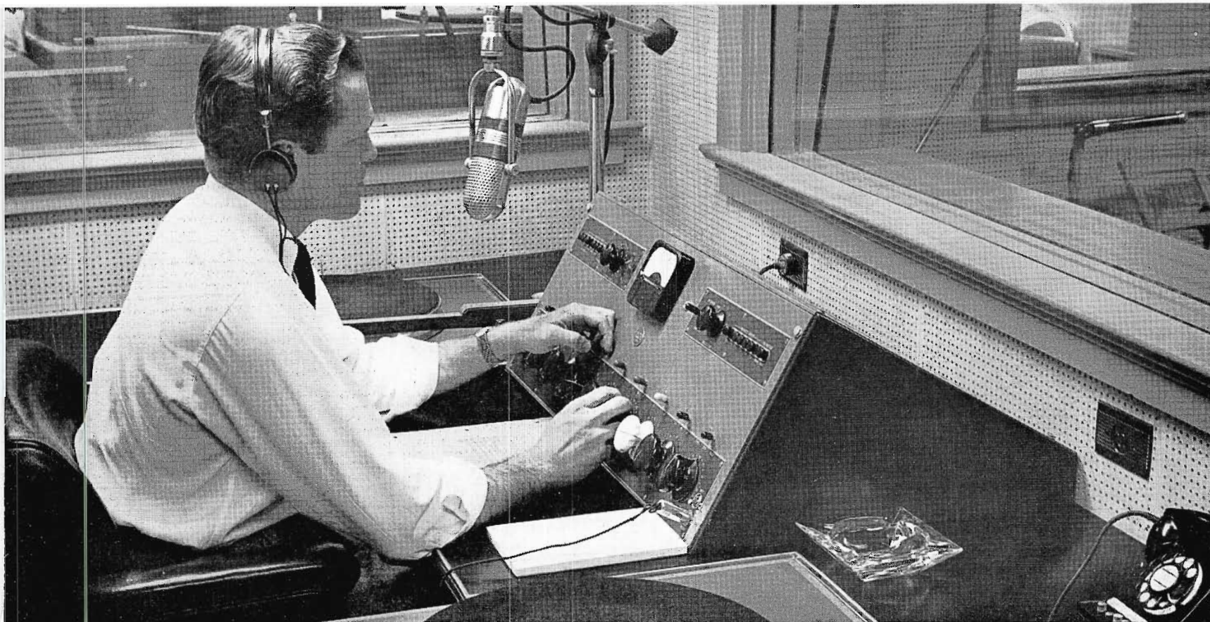
FIG. 8. "B" control room is, in effect, the center of operations, with its BC-2B console. Through the window to the right—partially visible—is the small speech studio and Control Room "C". Beyond the announcer is the recording room.
