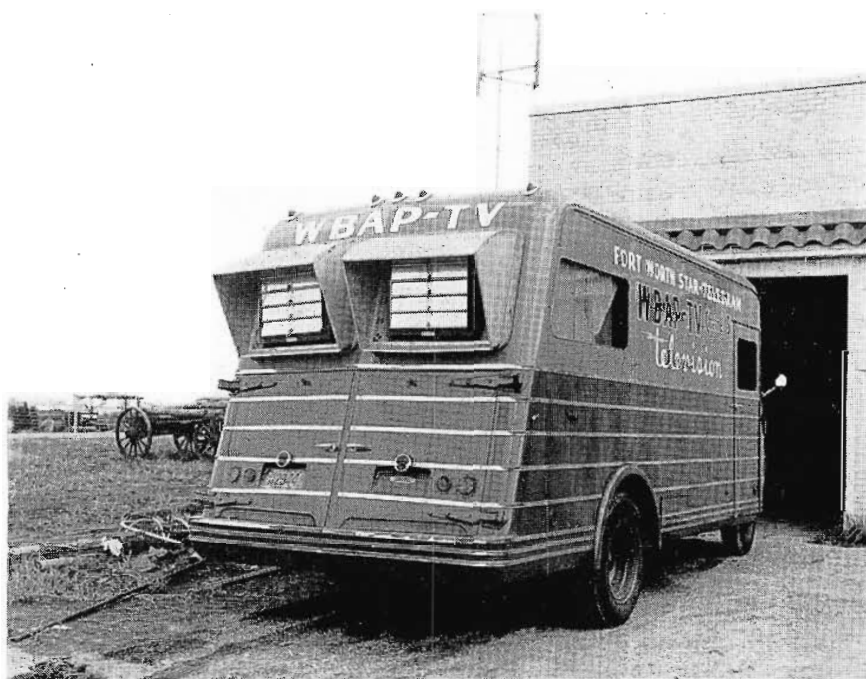
FIG. 22 (below). WBAP engineers have made a number of modifications in the TV-50A, most important of which is the addition of ventilating blowers. These were mounted in the rear windows as shown in this view. On a hot summer day this is much appreciated. Another modification provides for operation of four cameras instead of the usual three.
